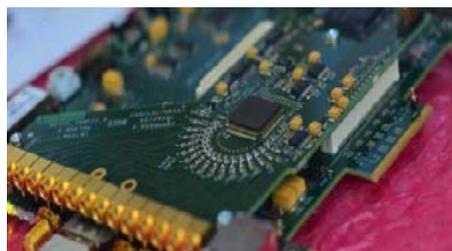
At the heart of the new AGILE telescope is the SAMPIC chip, which provides fast sampling, low power consumption, good radiation tolerance and built-in data reduction. (Courtesy: Christophe Royon)
