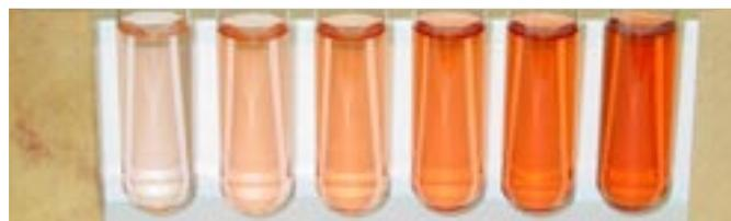
**Figure 4.** Blood-red coloured solutions produced by the ferric thiocyanate complex ion ( $\text{Fe}[\text{SCN}]^{2+}$ ). These solutions were prepared using the following range of  $\text{Fe}^{3+}$  standards: 2, 4, 6, 8, 10,  $12 \times 10^{-5} \text{ mol L}^{-1}$ .
