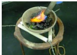
**Figure 1.** Set up used for heating a silverbeet sample in a crucible.
