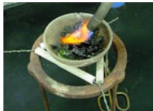
**Figure 1.** Set up used for heating a silverbeet sample in a crucible.
