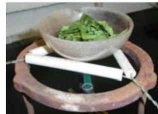
**Figure 2.** Set up used for combusting a silverbeet sample directly in the bunsen burner flame.
