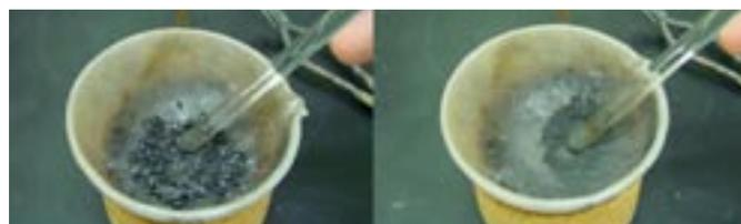
**Figure 3.** Left photo: ash remaining after combustion of a silverbeet sample. Right photo: silverbeet ash which has been ground to a fine powder using a stirring rod.
