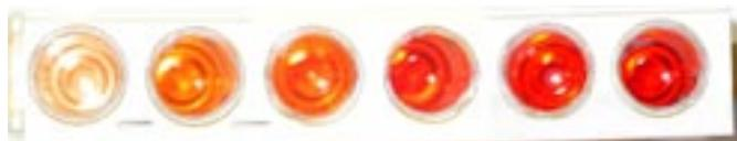
**Figure 5.** The same boiling tubes as in Figure 4 (prepared using  $\text{Fe}^{3+}$  standard solutions with concentrations of  $2 - 12 \times 10^{-5}\text{ mol L}^{-1}$ ) viewed from above, looking directly down the length of the tube. This view provides the most accurate "eyeball" comparison of the solutions' colour intensities.
