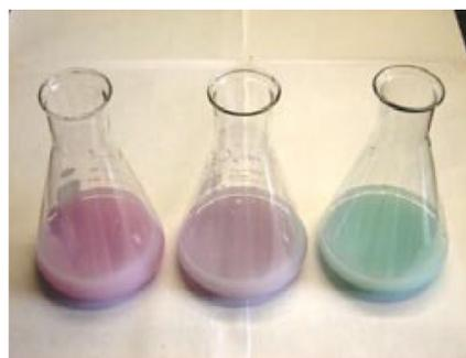
**Figure 2** Same colour changes for calcium-EDTA titration as in Figure 1, but for cloudy (opaque) sample solution, eg milk. Left flask: pink/red colour well before endpoint. Centre flask: last trace of purple colour just before endpoint. Right flask: blue colour at endpoint
