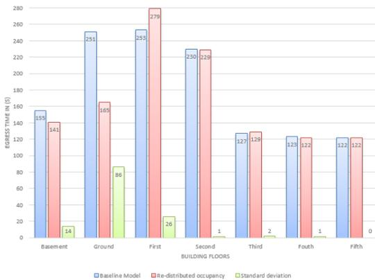
Figure 11 – Comparison of the building egress with different occupancy distribution in (s), mean and standard deviation
