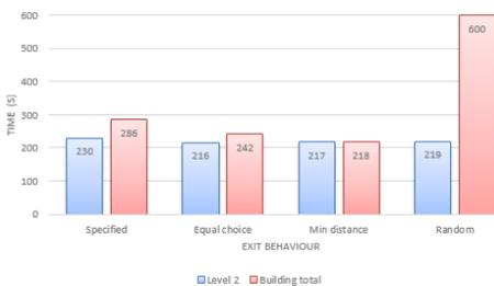
Figure 12 – Comparison of the evacuation time with various exit behaviours
