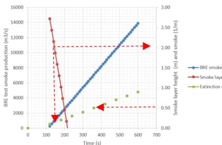
Figure 6 - Estimated smoke production, smoke layer height, and extinction coefficient
