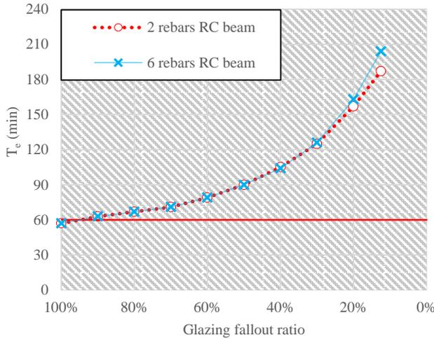
**Fig. 7** Impact of varying glazing fallout on minimum FRR values for RC beams for the C/VM2 60 min design scenario.
