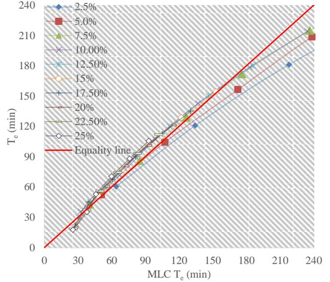
**Fig. 8** Comparisons of the C/VM2 method and the MLC method at various vertical vent ratios ( $\alpha_V$ ).
