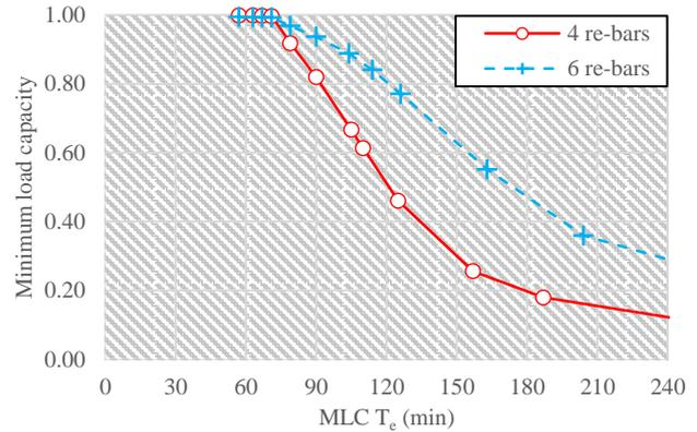
Fig. 11 Minimum load capacities attained by the two RC beams.
