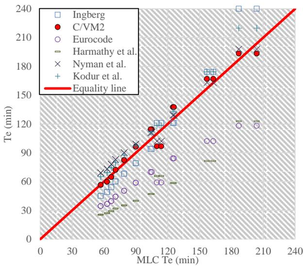
Fig. 4 Comparisons for the RC beams.
