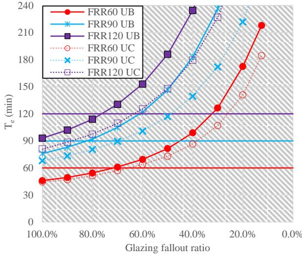
**Fig. 6** Impact of varying glazing fallout on minimum FRR values for the protected steel beam and column.
