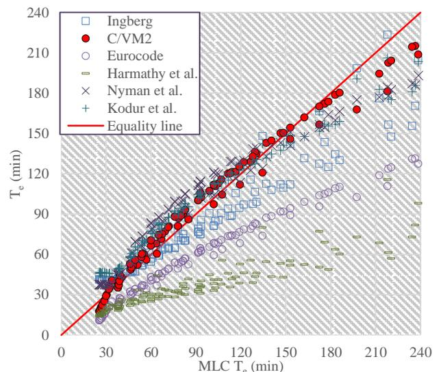
Fig. 2 Comparisons for the protected steel beam UB305 $\times$ 127 $\times$ 48.
