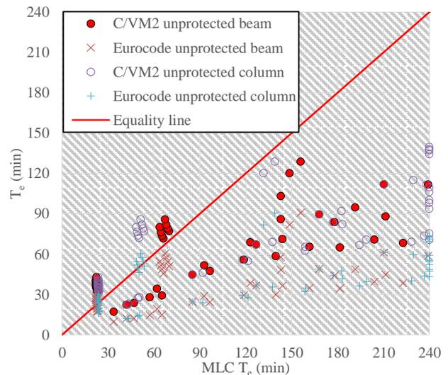
Fig. 5 Comparisons for the unprotected steel beam and column.
