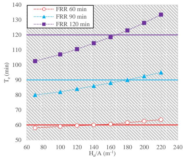
**Fig. 9** Impact of varying member size of protected steel beams on minimum FRR values.
