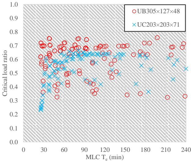
Fig. 10 Critical load ratio for the protected steel members.
