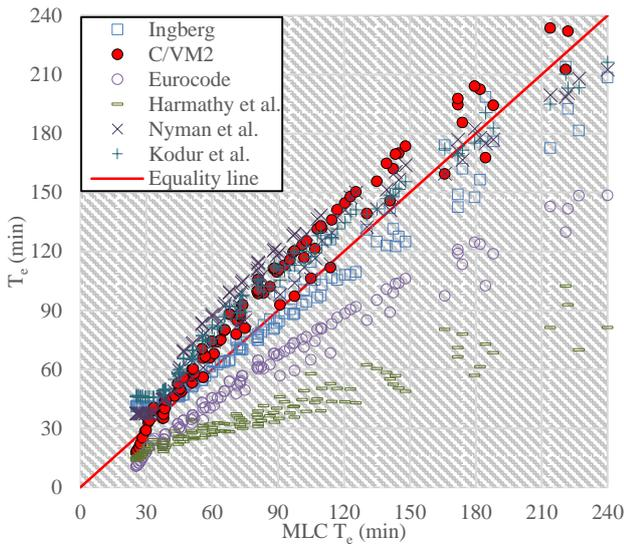
Fig. 3 Comparisons for the protected steel column UC203x203x71.
