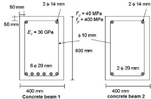
Fig. 1 Concrete beam cross-sections.
