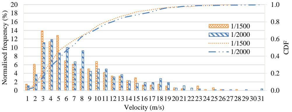
Figure 6: Droplet velocity distribution at position C with 3x magnification (37 kPa)
