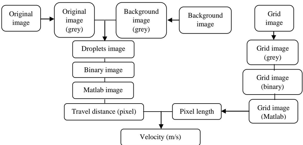
Figure 4: Flow chart for image processing
