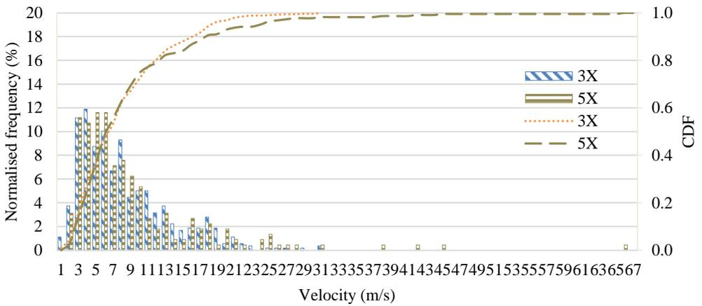
Figure 7: Droplet velocity distribution at position C with 1/2000 shutter speed (37 kPa)
