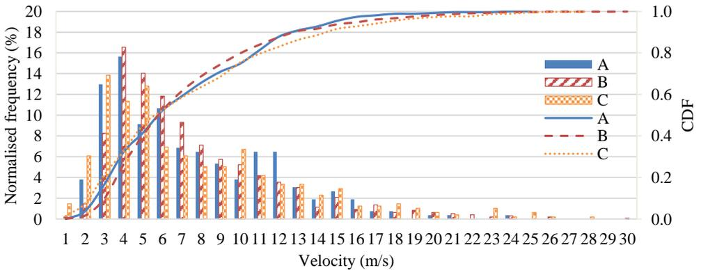
Figure 8: Droplet velocity distribution with 1/1500 shutter speed and 3x magnification (37 kPa)
