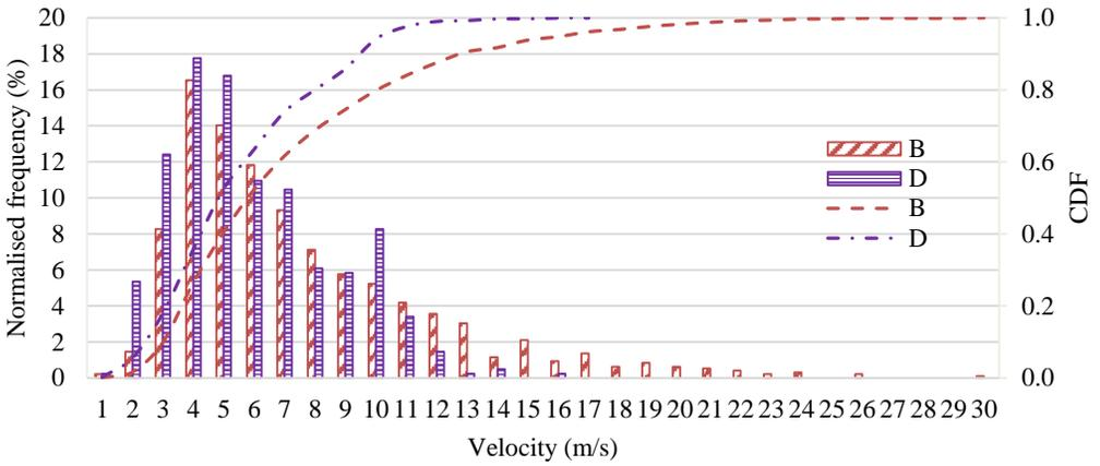
Figure 9: Droplet velocity distribution with 1/1500 shutter speed and 3x magnification (37 kPa)
