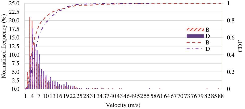
Figure 10 (a): Droplet velocity distribution with 1/2000 shutter speed and 6x magnification (88 kPa)
