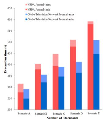
Figure 7: Evacuation time (s) comparison incorporating pre-evacuation times.
