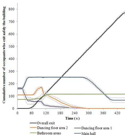
**Figure 15:** Average cumulative number of occupants that have exited the building for the EvacuatioNZ modelling of the Kiss nightclub fire with a total of 1,029 occupants.
