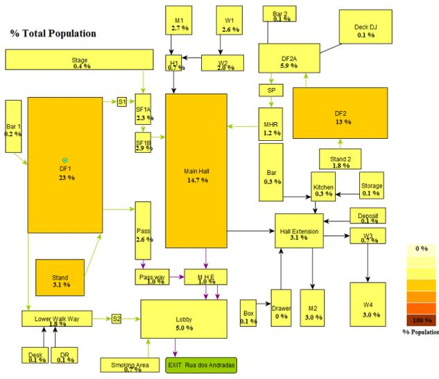
Figure 11. NFPA Journal model set-up in yEd graph interface.
