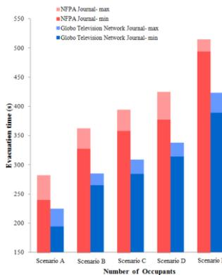
Figure 6: Evacuation time (s) comparison incorporating occupant characterization.
