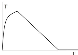
Figure 2 Typical shape of Eurocode Parametric fire [5]
