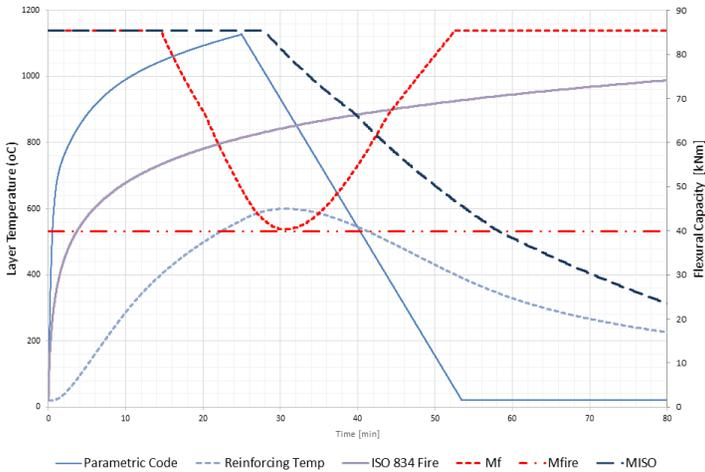
Figure 6 Eurocode fire, ventilation factor 0.2, 20 mm cover
