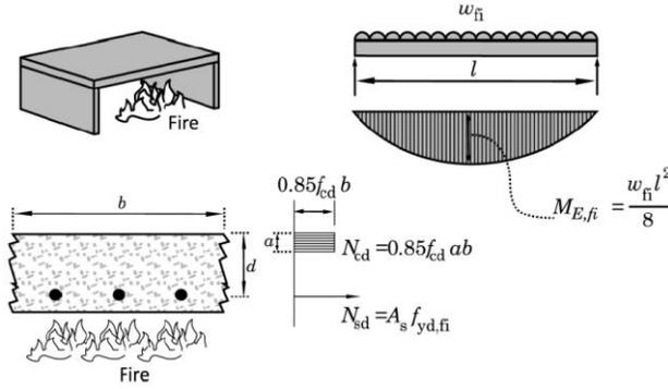
Figure 4 Simply Supported slab exposed to fire [5]
