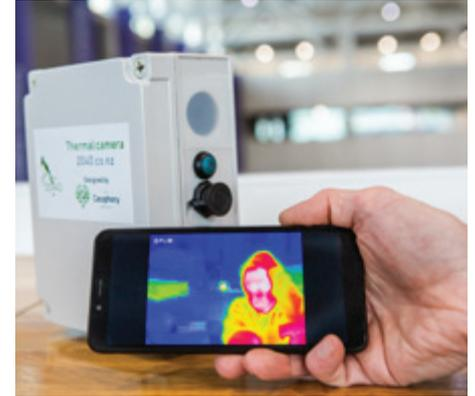
An image from the camera: to the left of the person's face, the bright circle is the constant-temperature plate of the calibrator
