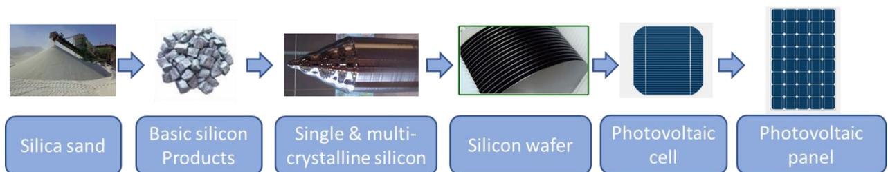
Figure 1 Basic process for silicon panel manufacture.
