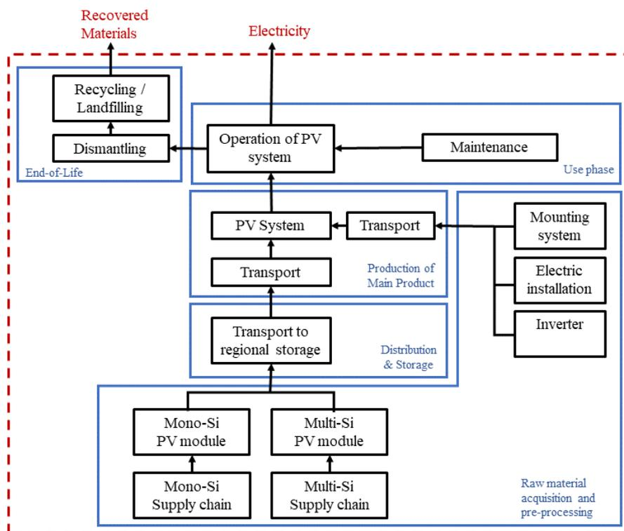
Figure 2 PV systems, showing the system boundary for considered activities, adapted from [1].
