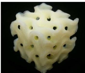
Gyroid triply periodic minimal surface lattice made by 3D printing
