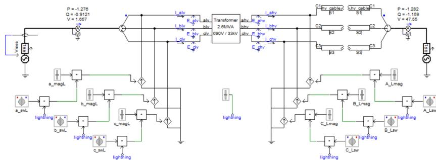
Figure 1. Transformer Model and Lightning Simulation.
