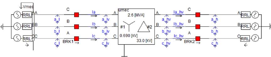
Figure 2. Switching Overvoltage Simulation.
