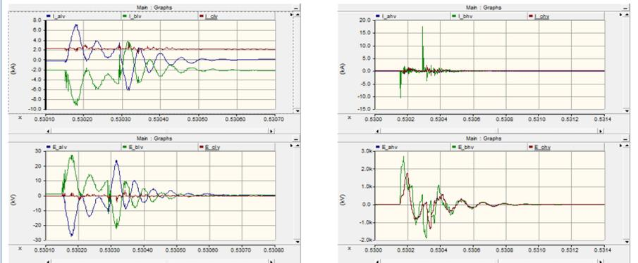
Figure 3. Lightning Response (LV response on left, HV response on right).
