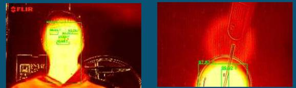
Identify the temperature of objects in the image and alert if the temperature  $> 38.3C$
