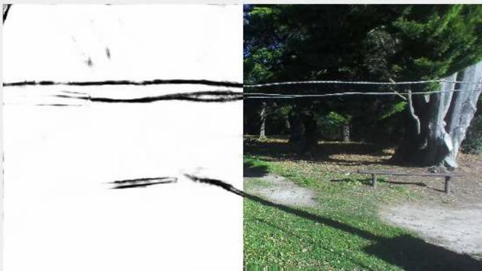
Fig 2. Sample edge detection (left) and input frame (right).
