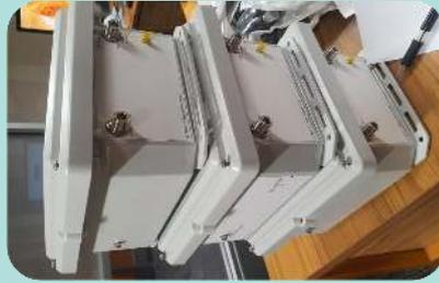
Four Zone Anchors (nodes) need to be built and set up around the campus to create a Trust Zone that can detect mobile nodes in an area. The materials to build these were sent from Foam and built at UC. These nodes took several weeks to build and took the most time to get working.
