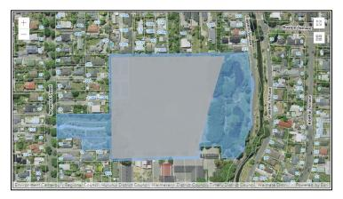
**Figure 12**: Contaminated (grey) and uncontaminated (blue) areas of Beckenham Park. The nature of the contamination is 'persistent pesticide bulk storage or use' (Environment Canterbury, 2021).
