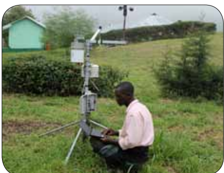
Cover Photo: Usman downloading data from one of the Hobo portable weather stations.
