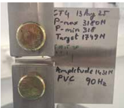
Test setup and 304/304L Compact Tension (CT) specimen
