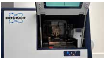
Bruker Dimension IconIR - Atomic Force Microscope (AFM) used for the research
