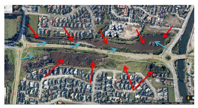
Fig 7. Probable stormwater runoff flow direction.
