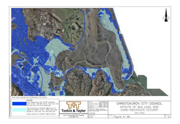
Figure 1: Projected inundation due to sea level rise and 1% AEP inundation event around Avon-Heathcote Estuary, Christchurch.
