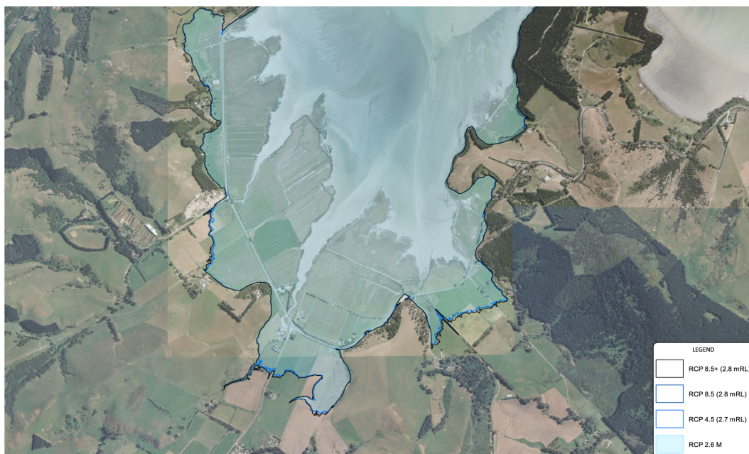
Figure 6. Inundation in Teddington for the year 2065. Created by Tonkin+Taylor (2017) for the Christchurch City Council Coastal Hazard Assessment. RCP (Representative Concentration Pathway) are alternative emission scenarios used by the IPCC. Date retrieved 18/10/2021.
