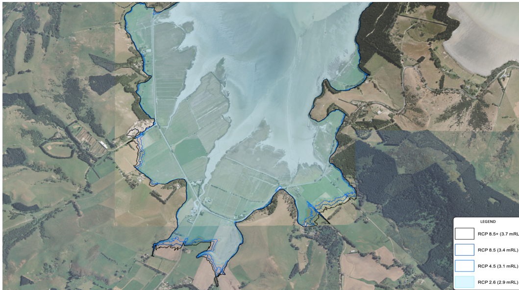
Figure 7. Inundation in Teddington for the year 2120. Created by Tonkin+Taylor (2017) for the Christchurch City Council Coastal Hazard Assessment. RCP (Representative Concentration Pathway) are alternative emission scenarios used by the IPCC. Date retrieved 18/10/2021.
