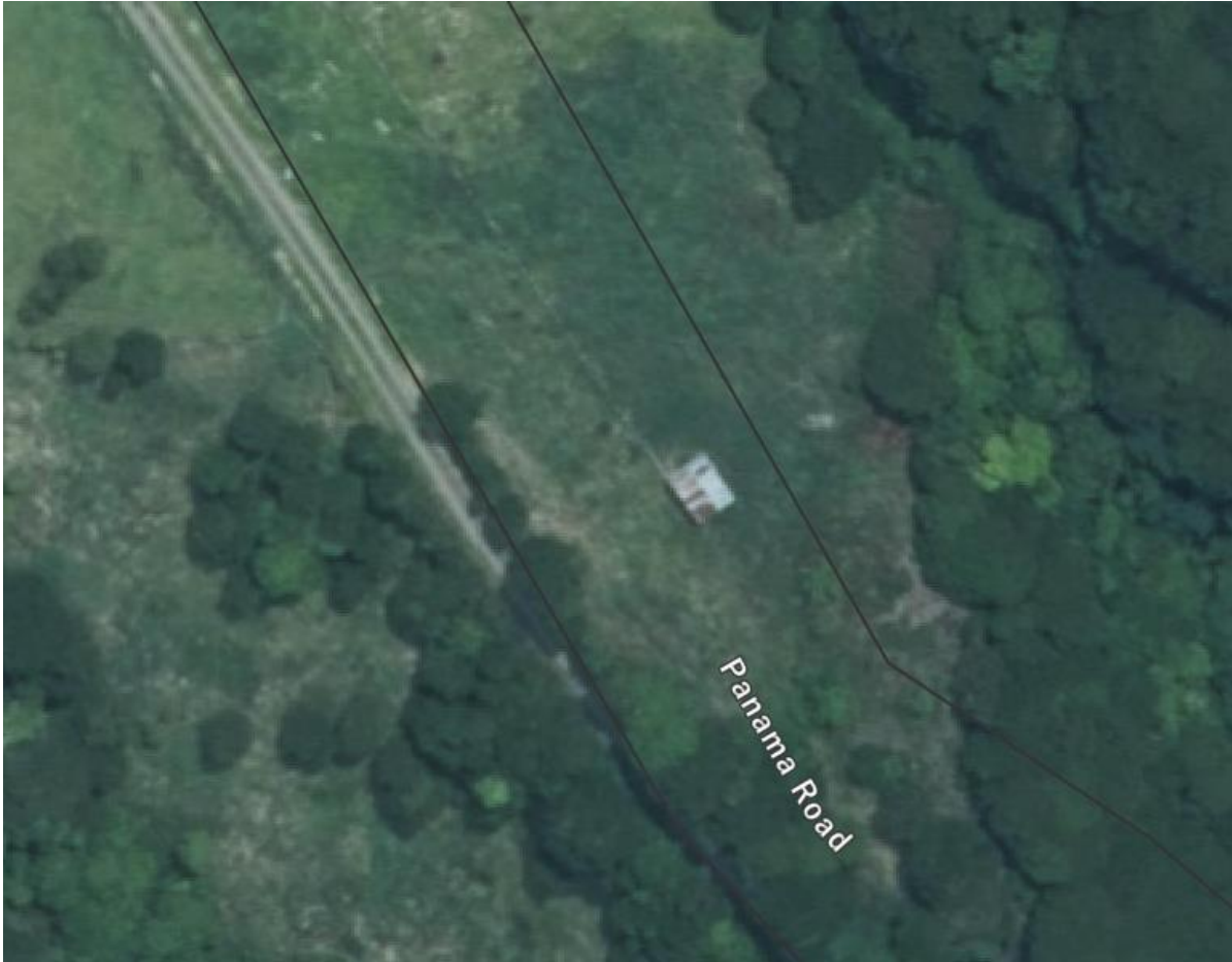
Figure 11: Council and PRR reserve boundary from historical land surveys. The council road boundary is offset from its actual position, highlighting the lower car park is predominantly on Council Land.
