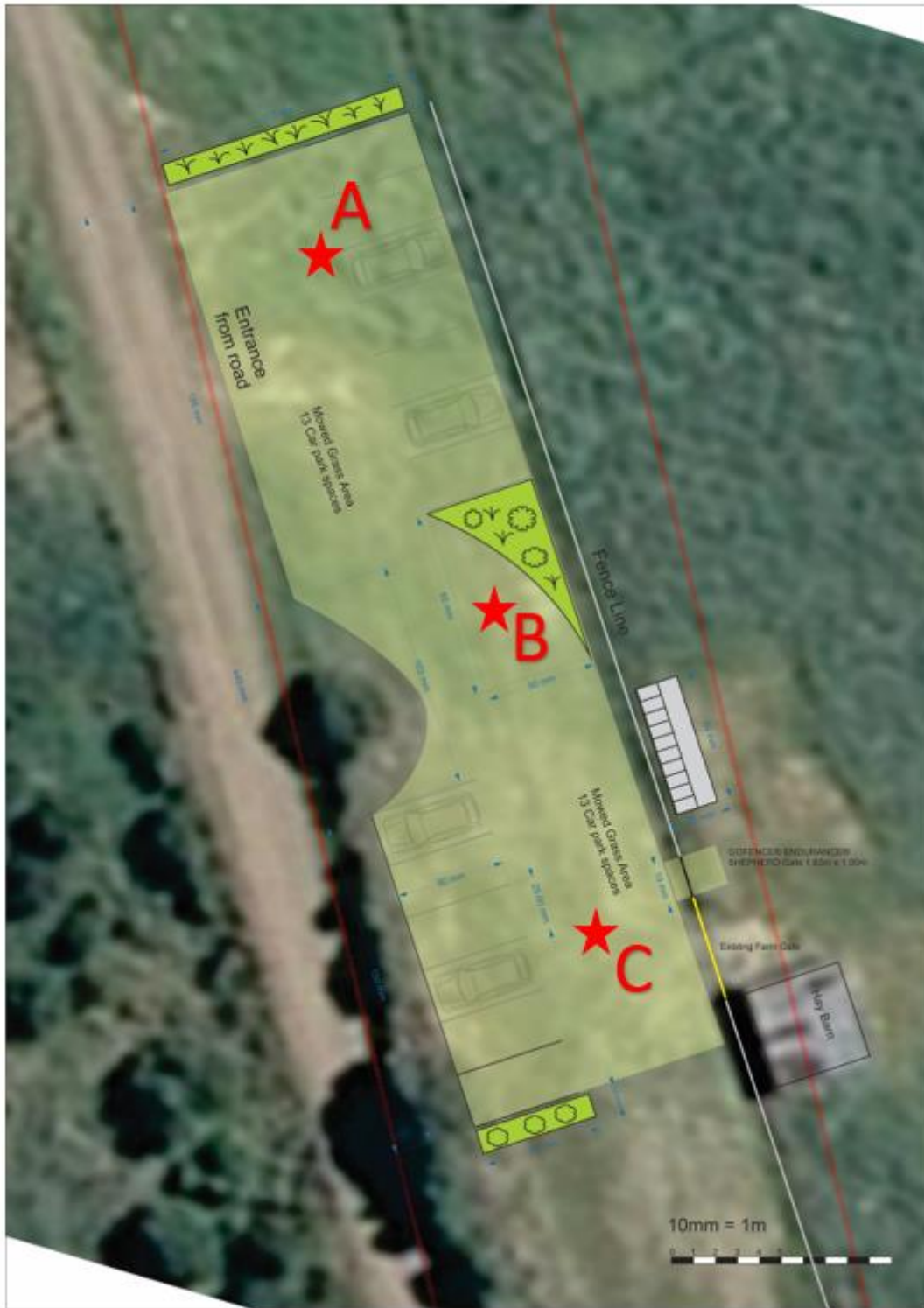
Appendix 3a: Lower Carpark testing locations for hand auger and scala cone penetrometer
