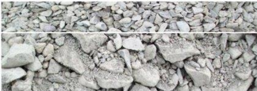
Figure 18: Cross section of AP65 and AP30 aggregate for proposed upper car park
