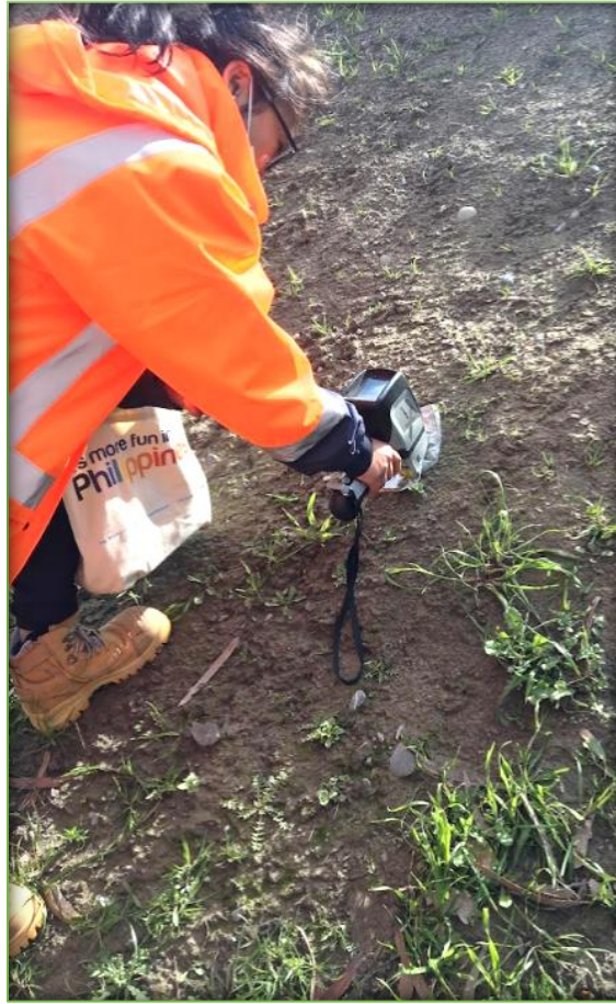
Figure 3. Soil testing at site 'one' with an XRF.
