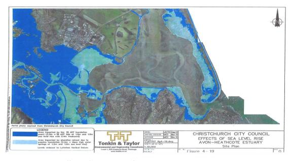
**Figure 1:** Predicted effects of sea level rise for the Avon-Heathcote estuary - 100 year projection. The light blue represents passive inundation, and the dark blue represents extreme inundation. Note. From Effects of Sea Level Rise for Christchurch City by Tonkin & Taylor Ltd, 2013, Christchurch City Council, p.63, (T&T Ref: 61707).
