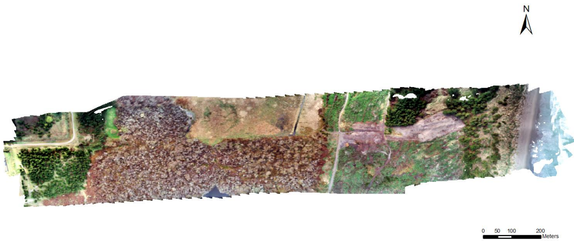
Figure 4: An orthomosaic image of the transect area produced in Agisoft Metashape.
