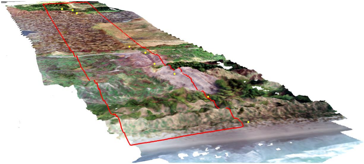
Figure 7: The final 3D model of the transect region, with the yellow points representing the locations of the soil samples. The forefront on the image is East, while the landward end of the transect is West.
