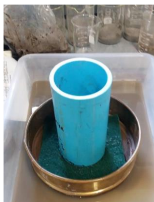
Figure 6: The setup of the permeability experiments; this photo shows the sand layer (sample c) being fully infiltrated after 31 minutes.
