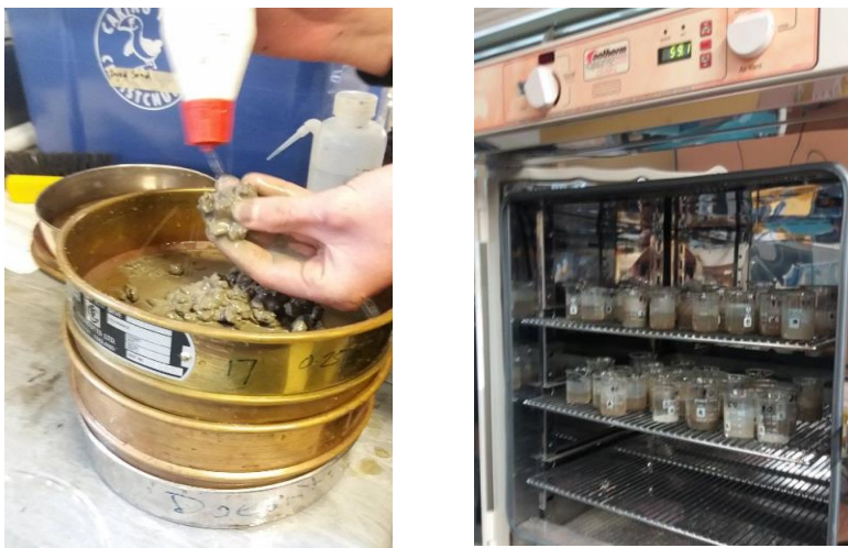
Figure 3: LEFT: Separating the clays and silts from sands gravels and pebbles by wet sieving; RIGHT: Samples placed in the oven to remove excess water before further analysis
