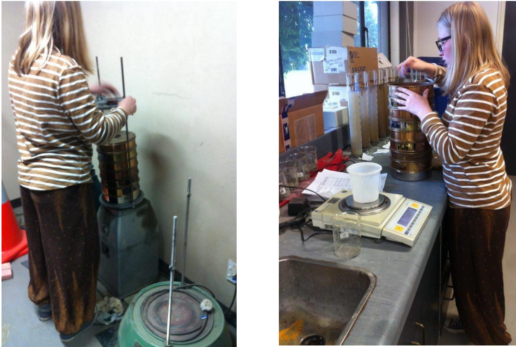
Figure 4: LEFT: Using the sieve shaker to sort the grain sizes in our sieves; RIGHT: Weighing the amount of sediment caught in each sieve size to get the amount of each corresponding grain size.
