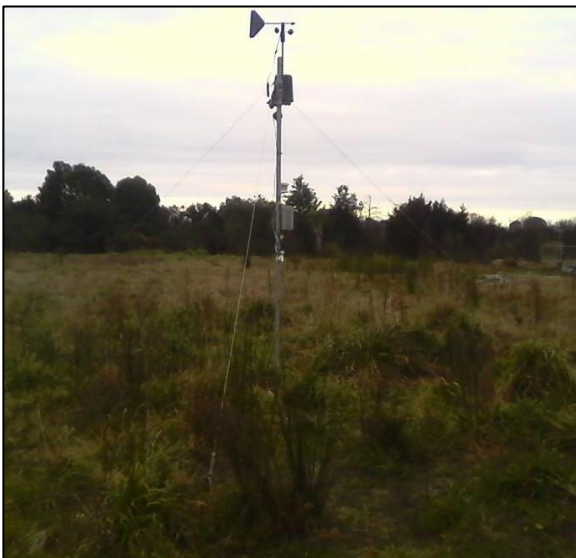
Appendix 4. The Onset Hobo H-21-001 portable Automatic Weather Station measured rainfall data.
