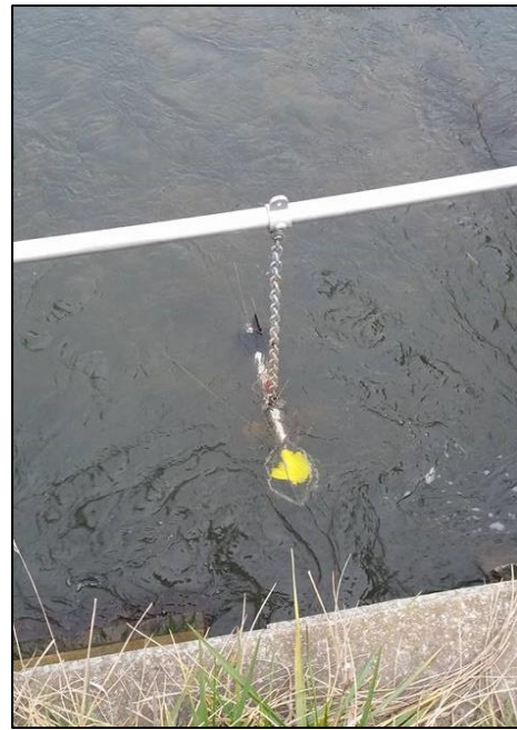
Appendix 3. Valeport 106 current meter was set up at the Lake Kate Sheppard culvert. In ten second intervals, the water velocity (m/s) and direction of water flow was recorded.
