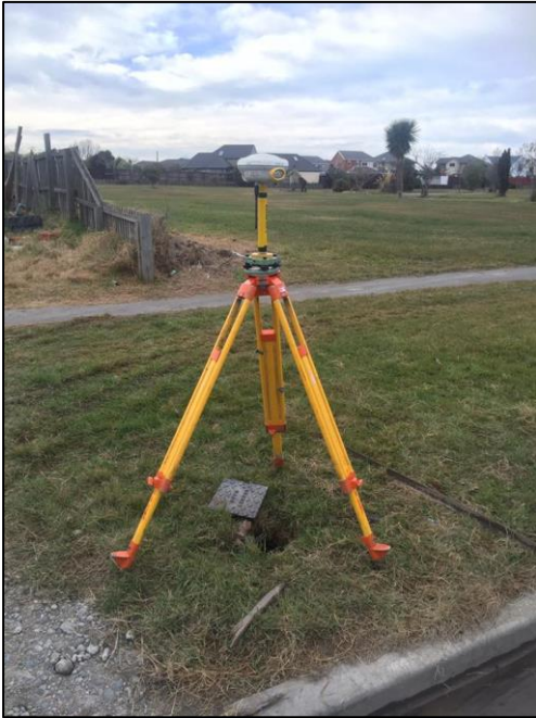
Appendix 2. Trimble R8 survey grade GNSS placed over a LINZ geodetic survey mark.
