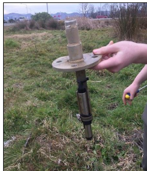
Appendix 5. The Solinst level logger 3001 used to measure conductivity, temperature and depth at 10 minute intervals.
