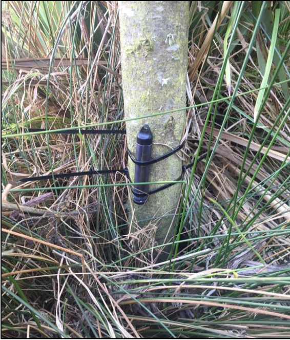
Appendix 6. The Barometric logger Solinst Barologger model 3001 measured air pressure. This was hidden amongst the riparian vegetation
