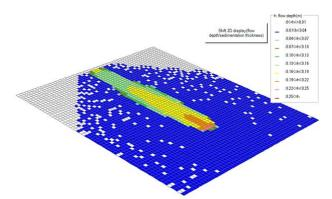
Figure 7 - Extent and depth of debris flow from main channel
