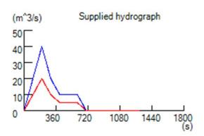
track. The scale of the debris flow modelled using default settings is much likely smaller than that of a potential debris flow from the yellow creek fan, the sediment output over time shown here shows a maximum discharge of 40 cubic metres of sediment and water per second, a realistic debris flow event would likely have a higher discharge
