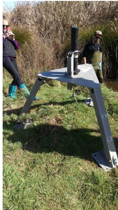
Appendix 2. The Acoustic Doppler Velocimeter (ADV) secured to a metal stand that was placed in front of the Travis Wetland Culvert.
