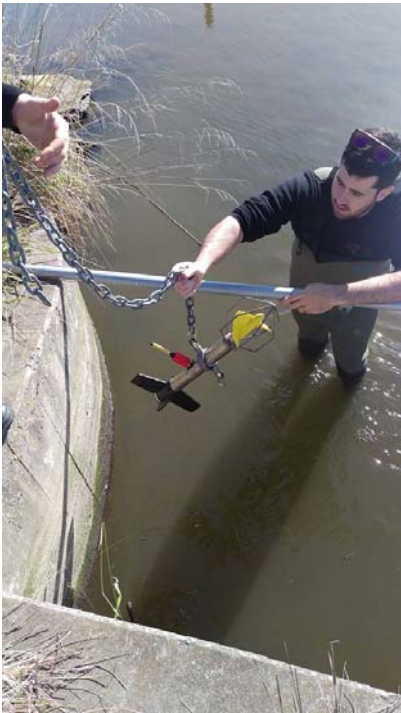
Appendix 1. The Nortek Valeport which is secured to a metal beam in front of the Avon River culvert.
