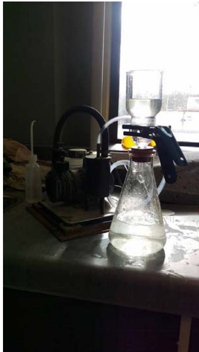
Appendix 3. One of the five sediment samples being processed through the filtration system.
