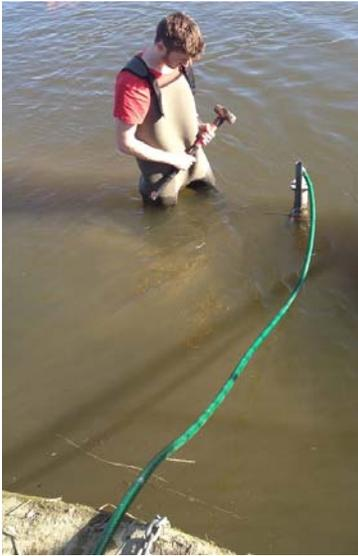
Figure A.4: An Odyssey CTD logger was used to measure continuous data however due to misinterpreted lag times the equipment was not installed at true low tide thus the equipment was not placed deep enough and data wasn't collected at low tide.
