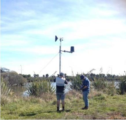
*Figure A.1. A requirement of the research was to record information before and after specific rainfall events. Therefore a weather station was positioned beside LKS to provide local meteoric conditions so the identification of these specific conditions could be made.*
