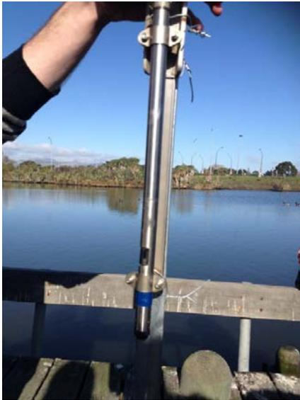
*Figure A.7: The CT2X logger that was stationed at the dock. This is the same unit that was damaged.*
