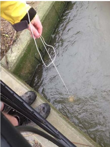
*Figure A.3: The use of a piece of string on the end of the RBR logger was used to lower the recorder into the water recorder the water profile at the given location. This was done at several locations throughout LKS, Travis wetlands and the Avon River.*
