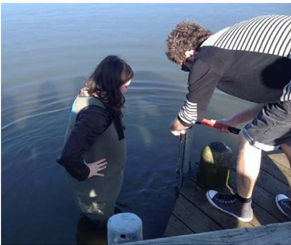
Figure A.5: Installation of the first CT2X logger beside the jetty in LKS. A waratah was driven into the lake floor with the logger secured to it. This provided reassurance that the logger won't move around, and makes it difficult for members of the public to interfere.
