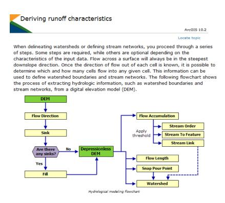
Figure D.2: Flowchart of steps taken in GIS drainage modelling
