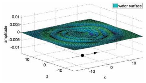
Numerical model results: 3D wave field generated by a submarine landslide. The landslide moves in the x-direction from the origin, indicated by the black circle. This generates the wave field shown.
