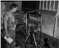
Geoff Merryweather observes flame spread tests over timber samples in the LIFT apparatus
