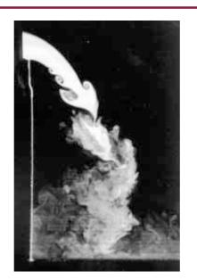
A salt water experiment to model smoke flow through doorways (invert picture - it looks like smoke)
