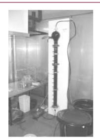
Fluidised bed reactor with coconut shells
