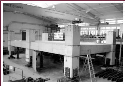
Test specimen ready for load frames to be attached
