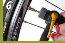
Before removing the pump, flip lever **DOWN TO UNLOCK**.
