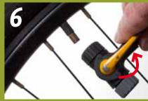
Before removing the pump, flip lever **UP TO UNLOCK**.
