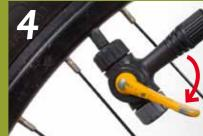
Flip lever **DOWN TO LOCK** it on, and start pumping.
