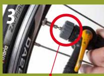
Attach the **GREY** coloured end Flip lever **UP TO LOCK** it on, of pump nozzle to valve.
