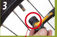
Attach the **BLACK** coloured end of pump nozzle to valve.
