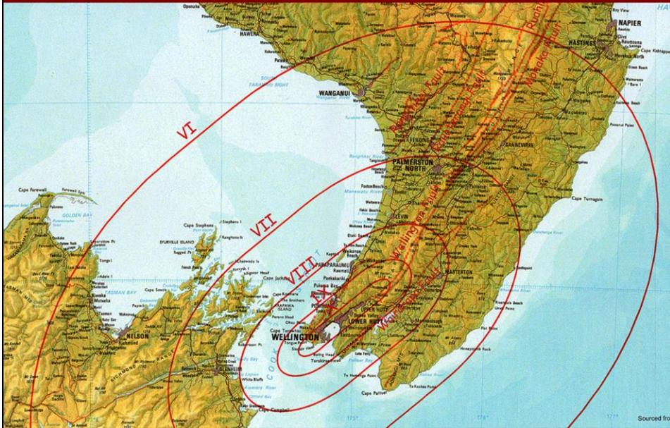
1. Application of GIS has provided the means to graphically display the earthquake risk to communities.
