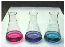
**Figure 1** Colour changes for calcium-EDTA titration in clear sample solution using Patton-Reeder indicator. Left flask: pink/ red colour well before endpoint (excess Ca<sup>2+</sup> ions present to complex with indicator). Centre flask: last trace of purple colour just before endpoint (Ca<sup>2+</sup> ions almost all complexed by EDTA). Right flask: blue colour at endpoint (all Ca<sup>2+</sup> ions complexed by EDTA, indicator completely uncomplexed).
