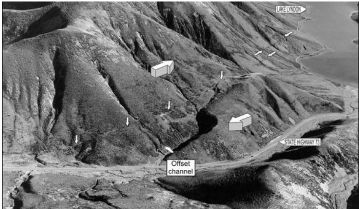
Figure 4. Oblique aerial photograph of Porters Pass fault between Porters Pass and Lake Lyndon facing south. White arrows show position of Porters Pass fault scarp, block arrows show lateral movement.
