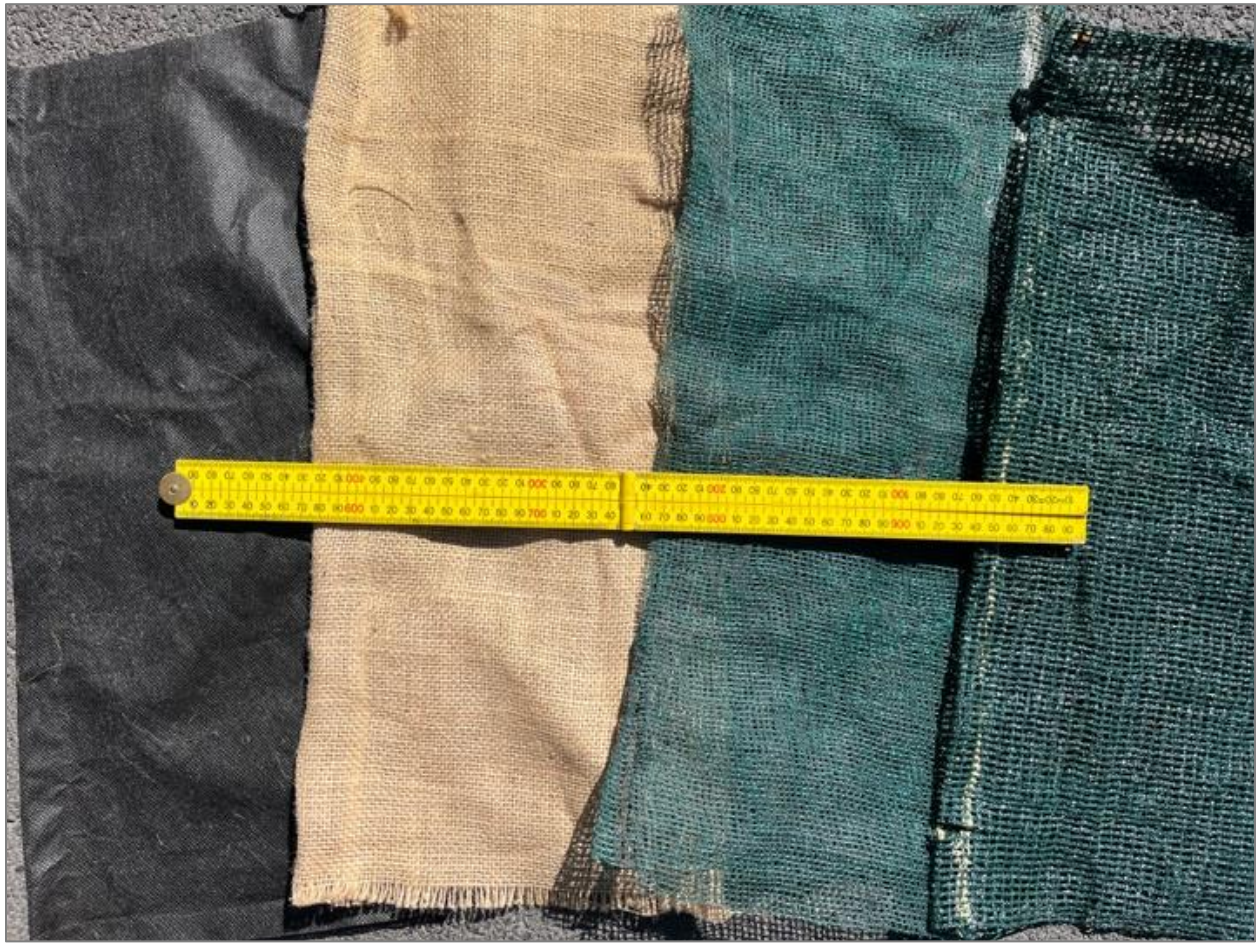
Figure 21: The materials used in the second controlled testing, including weed matting (left), hessian (middle left), finer shade sail (middle right), and shade sail with larger pores (right). A ruler shows their approximate pore sizes (Ferugson, 2025).
