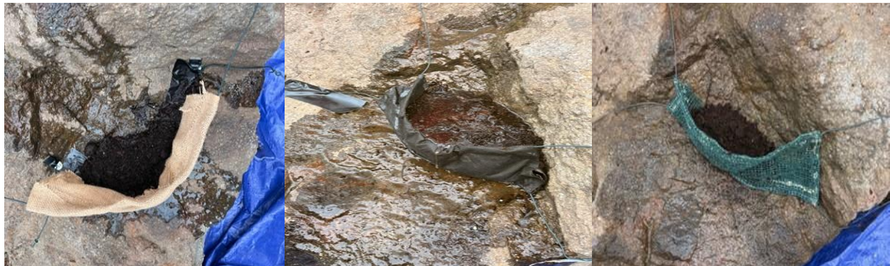
Figure 20: The hessian sling (left), weed matting sling (middle) and shade sail sling (right) during controlled testing (Ferguson, 2025).
