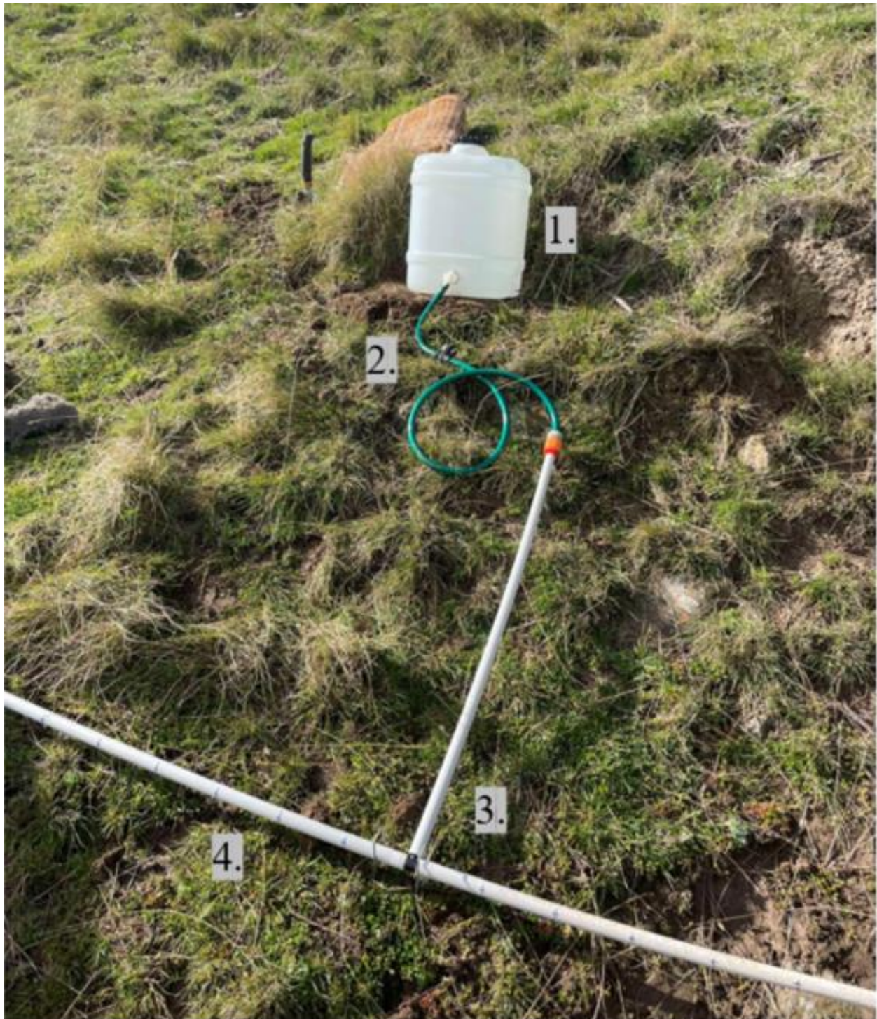
Figure 6: The water dispersal method. 1 = 20L water tank, 2 = hose connection, 3 = 4m spread tubing, 4= holes drilled 10cm apart spanning 1m (Bridgman, 2025).
