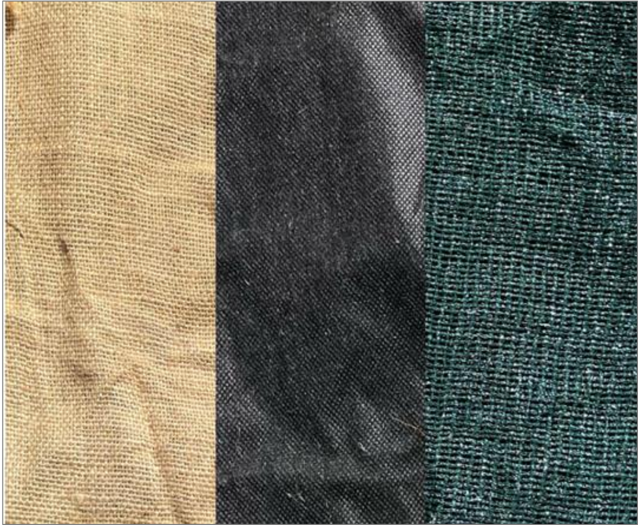
Figure 19: The three materials used in the first onsite field testing, including hessian (left), weed matting (middle), and shade sail (right) (Ferguson, 2025).
