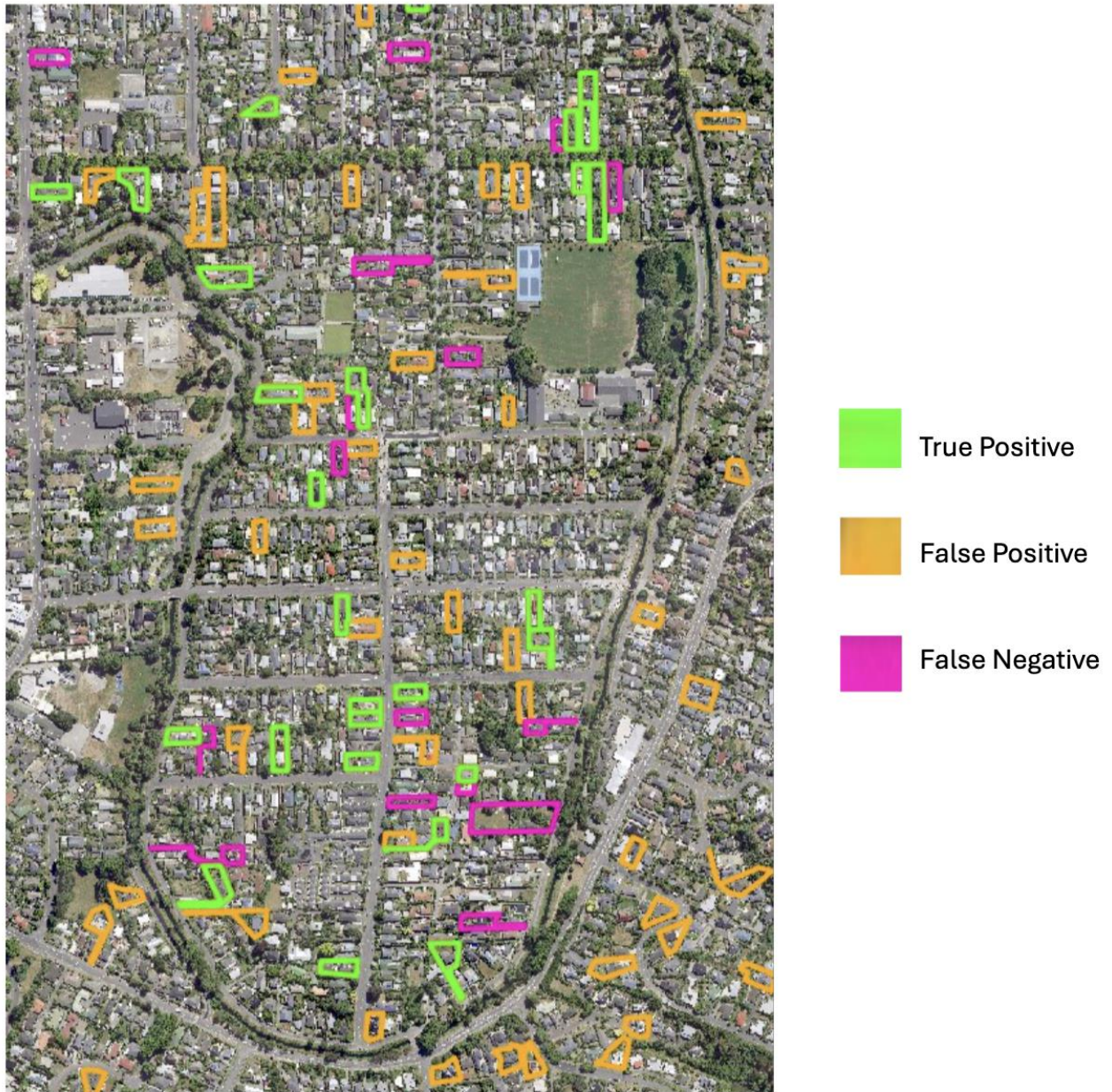
Figure 1. Map of Beckenham showing manual checks of solar panel detections. Green = true positives (manual + software detection), orange = false positives (software detection only), pink = false negatives (manual detection only). True negatives are not shown. Kappa index values were used to assess detection agreement.
