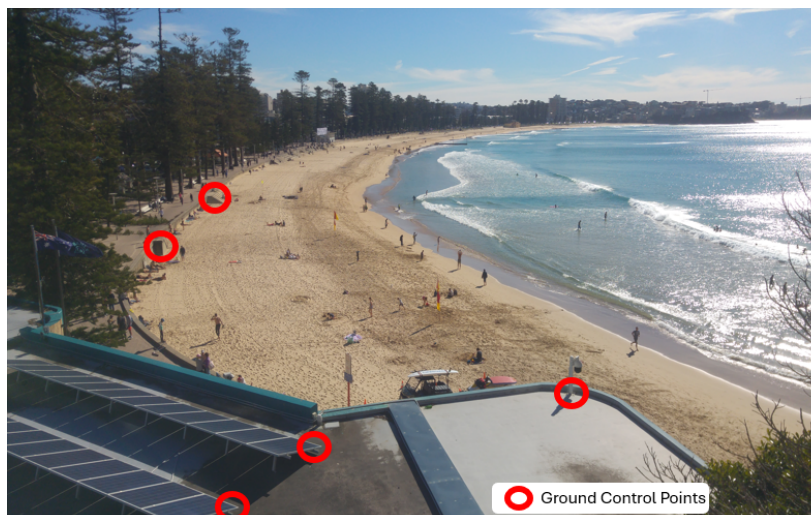
Figure 9: This image is an example of a good CoastSnap stands position. This stand is located at Manly Beach in Australia. Five fixed structures (marked in red circles) that won't change over time can be used for ground control points (used for image alignment). Adapted from the example CoastSnap image from the CoastSnap Starter Toolkit (Harley, n.d.).
