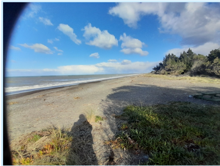
Figure 8: An example of an unusable image taken at Leithfield Beach using the CoastSnap stand. The edges of the image are distorted, compromising data quality.
