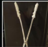
The poker tongs feature a simple design that allows the tongs to open and close with ease. Each end of the tongs is designed to be long enough where when closed, both handles hang inside and fold back. When in the open position, the tongs can act as a push and pull tool to be used for pushing logs.
