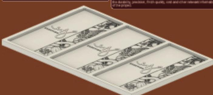
3D model of chocolate bar mould, manufactured via 3D print and made from PLA
