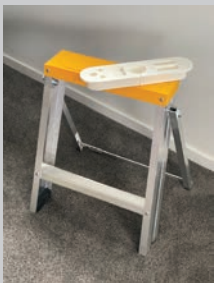
Figure 7: Prototype part of the ladder top frame and insert using 3D printing
