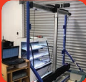
Experimental Set Up of traverse and data capturing equipment for HWA Testing
