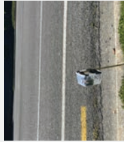
Figure 4. Arduino in position. Stakes were used to raise the boxes to increase recording reliability.
