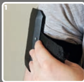
Attach the radio base plate to the arm using the velcro strap.
