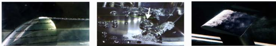
Figures 1-3: (Left) Tip vortex cavitation (TVC), (middle) travelling cavitation, (right) sheet cavitation.
