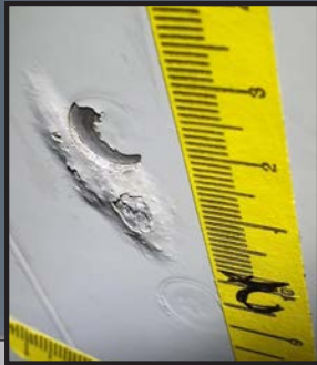
Fig 1: Corroded aircraft wing skin around fastener
