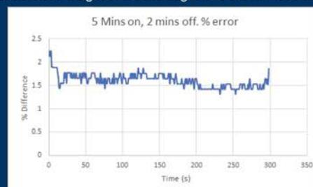
The graph shows the percent error of the data over a 300 second span. After around 30 seconds the graph stays in the region of around 1.5 -2% minimum value. The noise level was determined to be acceptable.
