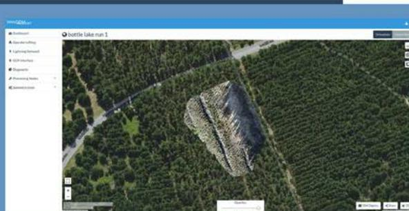
3 OpenDroneMap allowed for the creation of an ortho-tiff from the survey images. An ortho-tiff allows every pixel in the image to have a corresponding GPS coordinate. This meant that any wilding pines found in the image can easily be found by the spray drone from the GPS coordinates extracted from the ortho-tiff. This also allows this images to be overlaid on to google maps, which allows the user to gain a clearer understanding of where the survey is situated and how to get there.
