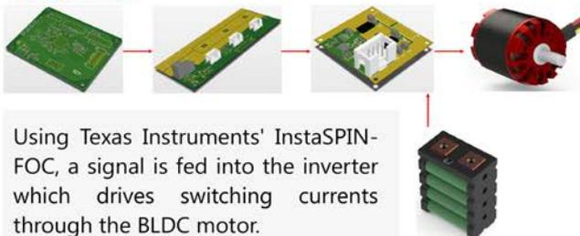
Using Texas Instruments' InstaSPIN-FOC, a signal is fed into the inverter which drives switching currents through the BLDC motor.
