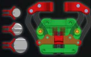
The grip mechanism to the left can be operated with 2 fingers, concentrically gripping dials strongly. When the red hub is pressed and released against the springs, the grips separate then close. Rubber grip surfaces maximise grip on a variety of dial shapes without damaging them.
