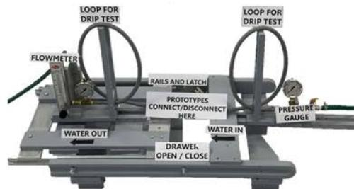
Figure 4 - Layout of test rig components
