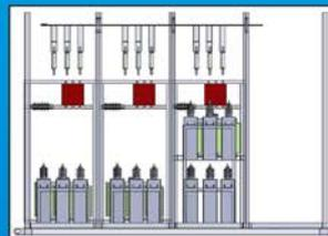
Figure 2: Interior of the enclosure showing placement of capacitor banks, vacuum contactors, detuned reactors, and main fuses. Enclosure is compartmentalised to protect equipment in case of a fault.
