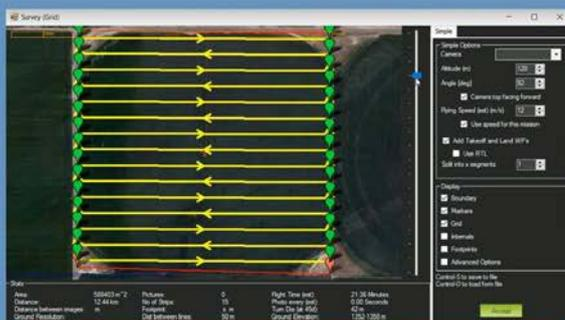
1 The first step in this process is to create a path for the UAV to follow. This was done by using ArduPilot. ArduPilot allows us to outline the area to survey on a Google maps like interface and it automatically creates a path that will cover the entire area. This is calculated based on the height that you want the drone to fly at, the camera that is on the drone and how much of an overlap that you want for the images.
