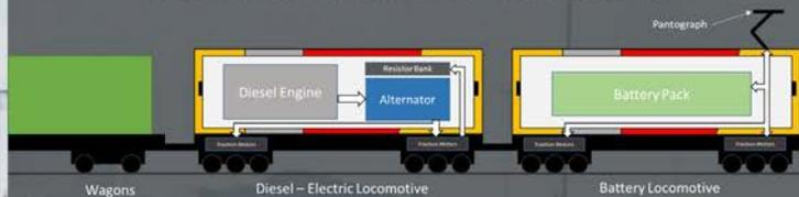
The hybrid system modelled in this project is a 'hybrid consist' - two locomotives, one of which is a conventional diesel-electric locomotive, and one which is powered through a battery and overhead lines. Both locomotives contain six electric traction motors which draw power from the power sources located in that locomotive. The simulation manages these sources to optimise locomotive energy use.
