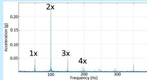
Effects of 50 Hz motor speed clearly evident.
