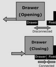
Figure 3 - Side view schematic of DishDrawer™. Top drawer shows the connection coming apart when opening. Bottom drawer shows the connection closed.
