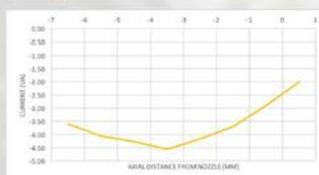
Water pressure of 5 bar, electrode voltage of 3 kV and a position of 3-4 mm between the electrode and the nozzle outlet gave maximum current of  $-4.5 \mu\text{A}$ .
