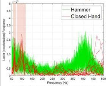
Figure 1: Frequency bands of hammer (handle) input and resonance of hand in grip position.
