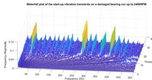
The VTV122 vibration transmitter consistently measured higher RMS vibrations for non-nominal test cases. Temperature sensors on both the bearing housing and the outer race were also indicative of irregularities when correcting for changes in the ambient temperature.
