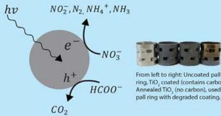
From left to right: Uncoated pall ring, TiO<sub>2</sub> coated (contains carbon), Annealed TiO<sub>2</sub> (no carbon), used pall ring with degraded coating.
