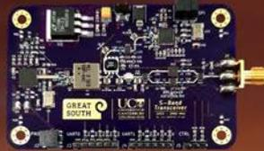
Figure 2 S-Band Transceiver
