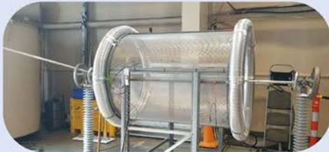
Ideal 220kV capacitor parameters depend heavily on the polarity of the streamer discharge process and the strongly non-uniform electric field strength on the curved tube edges.
