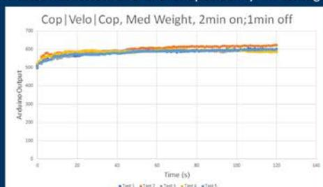
The graph illustrates the Velostat sensors repeatability and drift over 5 tests. Values converged to ~600 after 2 minutes. From this it was deemed that drift was not a factor at low time values and, that it was repeatable.
