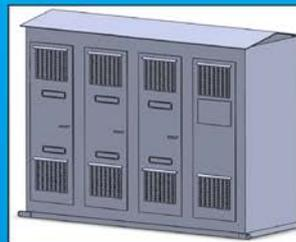
Figure 1: Enclosure designed to house the capacitor banks. The enclosure provides protection from arc-flash as well as a rating of IP55. Positive air pressure is maintained by an HVAC system to keep out contaminants such as dust.
