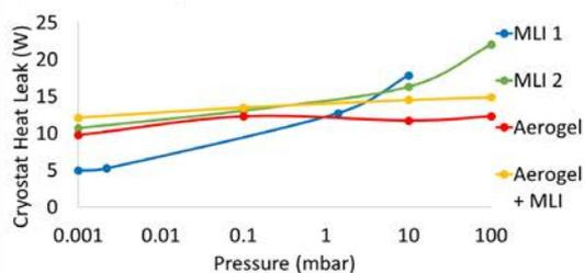
Figure 4: Heat leak of insulation materials at varying pressures
