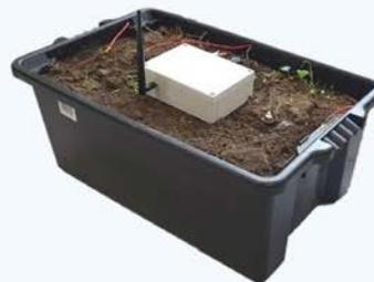
The test rig validates the functionality of the EFS by simulating earth faults. Mains voltage is applied through soil in a protective container where the EFS probes can be placed. A Variac is used to determine the fault voltage and a programmable relay sets the fault duration.
