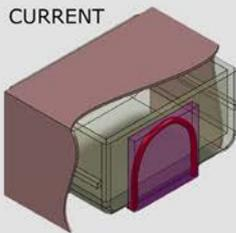
Figure 1 - Rear view of DishDrawer™ with tub exposed. Volume occupied by current link system shown in pink. Current Link hose shown in red.
