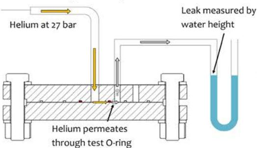
Figure 2: Set up of vacuum decay test rig
