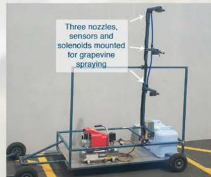
Three nozzles, sensors and solenoids mounted for grapevine spraying
