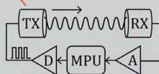
An MPU chip triggers a driver (D) to run TX. Propagation is measured from the amplified (A) return signal.
