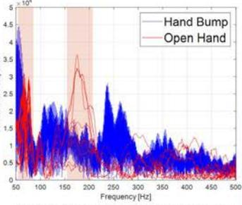
Figure 2: Overlapping frequency bands of hand bump (user testing) and resonance responses of the hand in an open position (lab testing).
