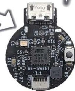
Figure 5: Glucose Sensor PCB
