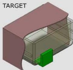
Figure 2 - Rear view of DishDrawer™ with tub exposed. Green volume shows the proposed area for the new solution.
