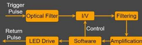
A surface mount LED pulsing at 5A is used to transmit infrared light back to the camera to indicate that the active target has been detected.
