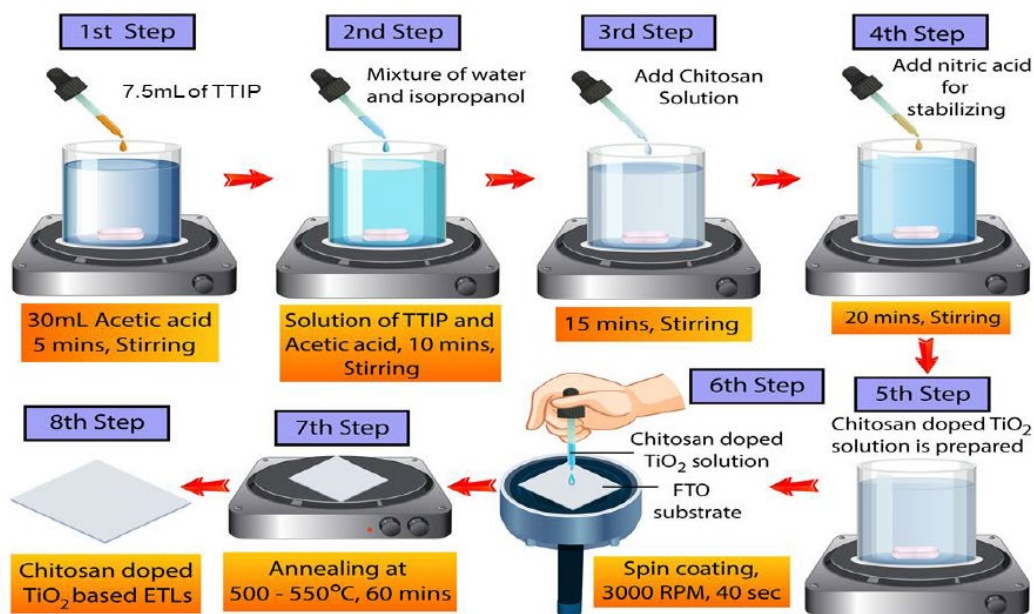
Figure 1. Schematic illustration of synthesis procedure of Chitosan-doped TiO 2 .
