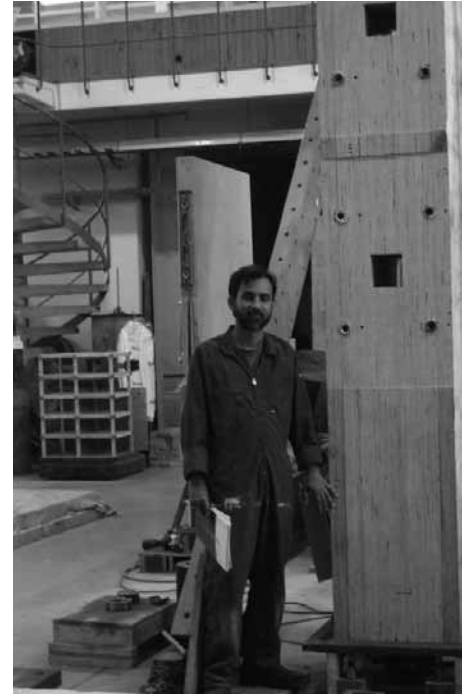
Full-size timber column tested by Asif Iqbal
