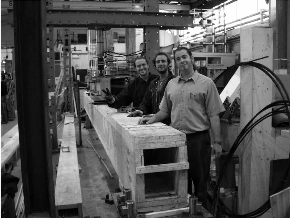
Long span prestressed timber beam tested by Claudio, Bruno, and David Carradine
