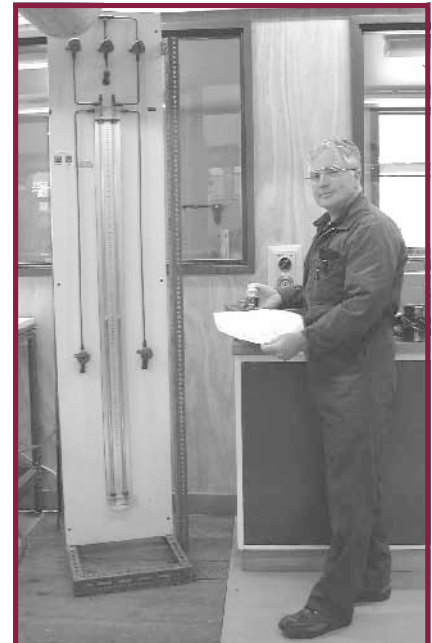
Ian Sheppard with a bottle of stored mercury. He is alongside a mercury filled manometer used in undergraduate laboratories.
