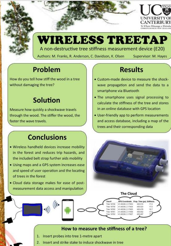
3. Device produces a tree stiffness measurement and stores it in an online data base with corresponding GPS coordinates
