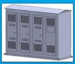
Figure 1: Enclosure designed to house the capacitor banks. The enclosure provides protection from arc-flash as well as a rating of IP55. Positive air pressure is maintained by an HVAC system to keep out contaminants such as dust.
