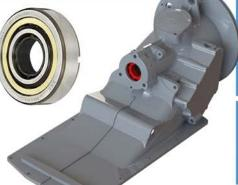
vibrations for non-nominal test cases. Temperature sensors on both the bearing housing and the outer race were also indicative of irregularities when correcting for changes in the ambient temperature.
