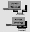
Figure 3 - Side view schematic of DishDrawer<sup>™</sup>. Top drawer shows the connection coming apart when opening. Bottom drawer shows the connection
