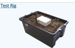
The test rig validates the functionality of the EFS by simulating earth faults. Mains voltage is applied through soil in a protective container where the EFS probes can be placed. A Variac is used to determine the fault voltage and a programmable relay sets the fault duration.
