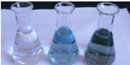
**Figure 1** Titration of a colour-free Vitamin C tablet.
