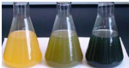
**Figure 3** Analysis of Vitamin C in freshly squeezed orange juice. Left flask: before the endpoint, the colour of the solution reflects the bright orange colour of fresh orange juice. Centre flask: Once all the ascorbic acid has been oxidised, a slight excess of added iodate forms a starch-iodine complex, a green colour in this case. This is the endpoint of the titration. Right flask: If further iodate solution were to be added after the endpoint.
